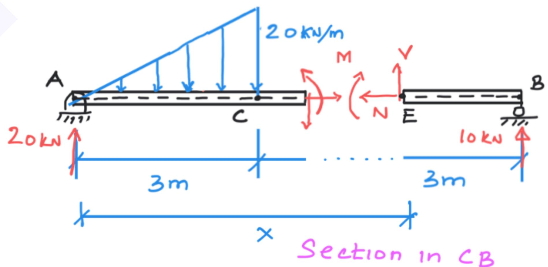
Step 2: Identify points of discontinuity and segments to consider, and develop math functions for  $V$  &  $M$  in each segment.
